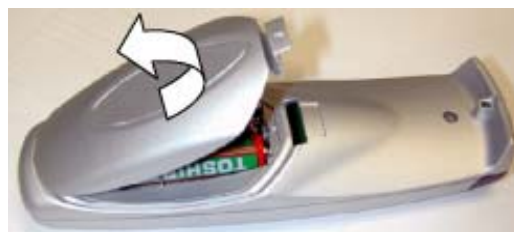
Image 8-2 Battery cover removal
