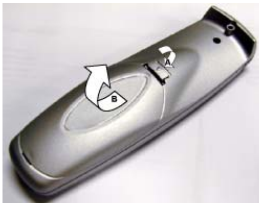
Image 8-1 Battery cover unlock
